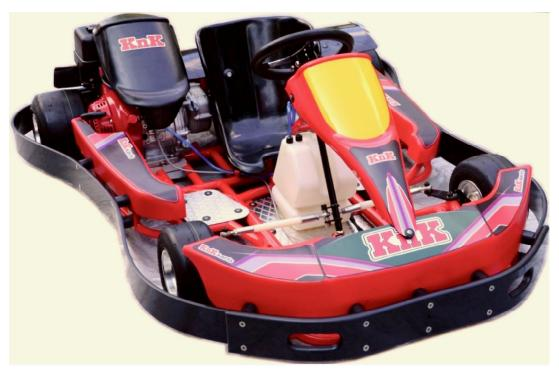
The Genesis SX3 is specifically designed for taking the abuse of high-speed tracks and heavy drivers. The main tube of the chassis is 32mm diameter steel alloy tube with a wall thickness of 6mm. A load distributing floating tube of 38mm with a wall thickness of 3mm supports the main tube, which permits chassis flex and rigid support at the same time. This strong middle section of the chassis prevents the chassis from bowing when impacted at high speeds.
